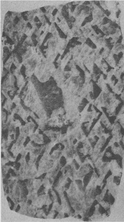
FIG. 2. Graphic granite, Jointora, Bihar, India. Ground on (100), showing local impoverishment in quartz. \times 2.5 .
