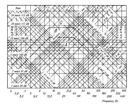
Vibration standards for main geared turbines, thrust bearings, boilers, heat exchangers, ICE-driven generators, shaff-generators, turbo-drives, turbo-generators and piston compressors
