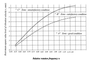
Fig. 9.9.3 Vibration standards of azimuth trusters
