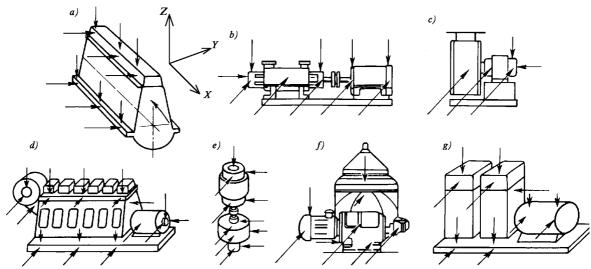
Fig. 9.2.5 Points of vibration measuring:
