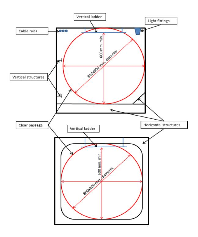
Fig. 4.5.5 Example of possible arrangements of escape fitted with a hatch taking into account minimum internal dimensions of clear width
