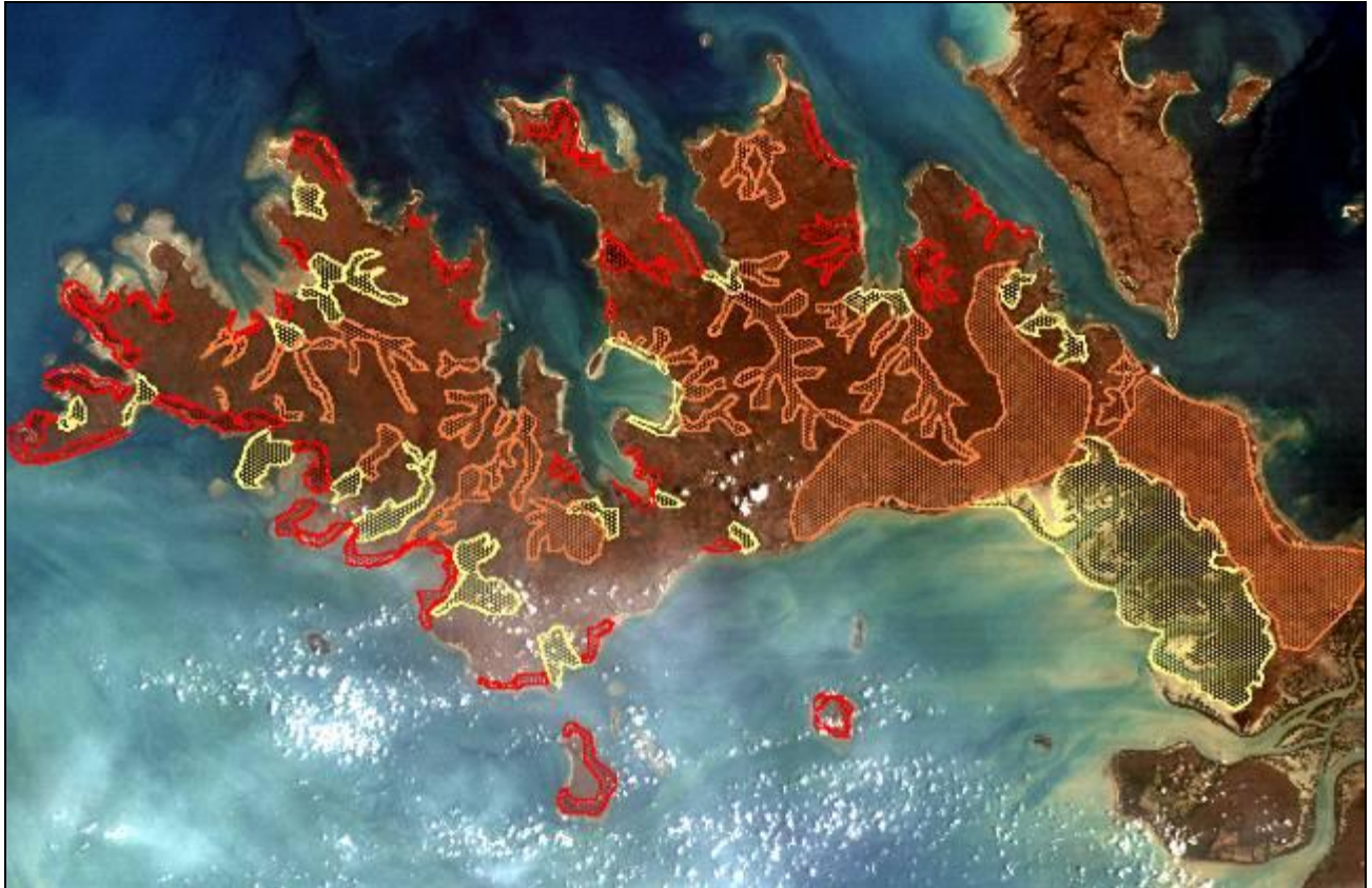
Figure 3-12 Classification of groundwater influences on wetland hydrology. Red corresponds to high levels of influence, orange is moderate and yellow is low (source: Geoscience Australia 2008)
