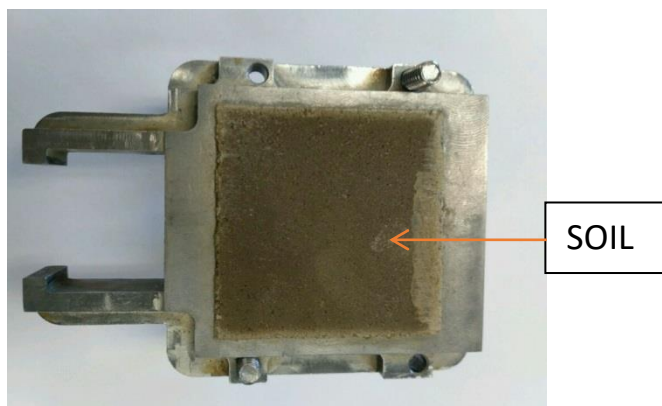
Figure 4.5 Upper part of the shear box with soil, a view from the top
