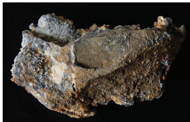
Figure 9. The reverse of Figure 8 (the upper side in the cavity) showing rock with a thin crust of pyrite and ‘ankerite’.
