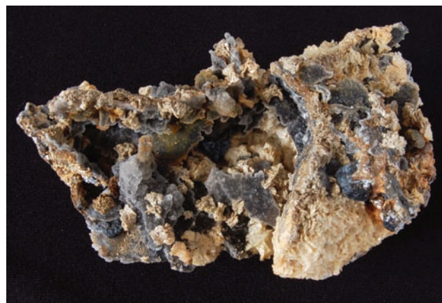
Figure 8. A specimen of ‘ankerite’ with quartz and minor sphalerite (the underside in the cavity). Specimen width 14 cm.
