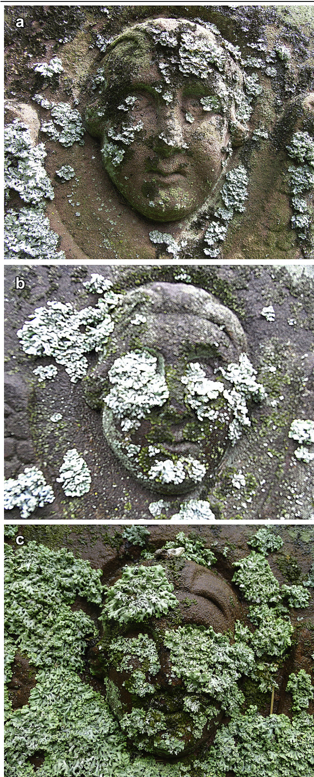
Fig. 10 – Lichens are important geochemical agents and oxalate is produced by many species, contributing to physical and chemical biodeterioration of the substrate. This can lead to profound changes that are especially evident in cultural heritage. The figure shows successive images of a gravestone taken over an approximate seven-year period, showing phases of lichen colonization and also areas of detachment of biomass with resulting loss of underlying substrate. Images recorded (a) 07.07.2007 (b) 23.01.2010 (c) 04.05.2014.
