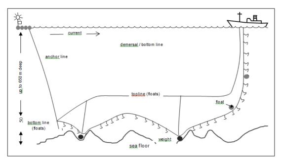
FIGURE 4-12: TYPICAL CONFIGURATION OF DEMERSAL (BOTTOM-SET) HAKE LONG-LINE GEAR USED IN SOUTH AFRICAN WATERS.
