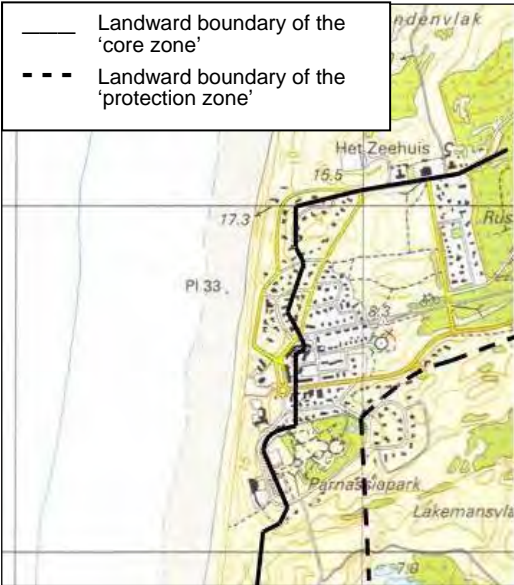
Fig. D-3.1: A coastal town under risk (source: Rijkswaterstaat (2005a)). Sea-side town in the Netherlands with coastal protection zonation (safety lines) that affects the regulations regarding land-use and activity allocation. In this area the flood protection is provided by coastal dunes. The zonation is hence derived from a safety assessment of coastal dunes based on storm erosion calculations and economic value under risk. The 'core zone' refers to the zone that is currently part of the coastal defense against flooding. This zone has no legal protection level with respect to coastal erosion or flooding. The 'protection zone' is the zone that may become part of the coastal defense zone in the next 200 years due to expected rise in sea level.
