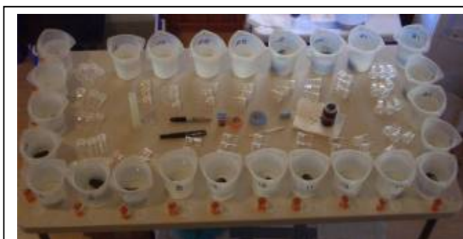
Figure 5. Clearance rates were measured by monitoring particle disappearance in beakers containing single mussels, relative to controls with no mussels.
