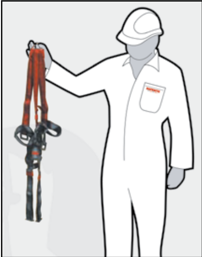
a. After carrying out an inspection of the harness hold the rear dorsal “D” ring and shake the harness and untangle all the webbing and unfasten all the buckles.
