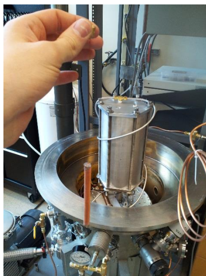
Figure 16: Image of the suspended catalyst dipper probe to ensure complete conversion to parahydrogen in the condenser.
