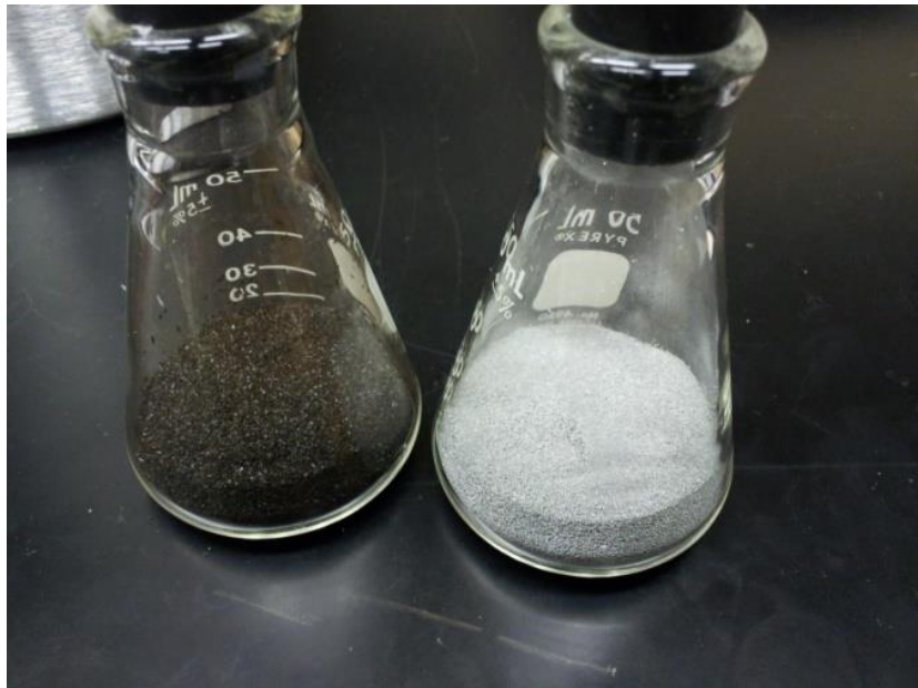
Figure 15: (Left) Ionex™ O-P catalyst compared with (Right) non-catalytic aluminum powder.
