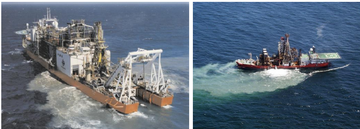
Figure 34: Typical crawler-vessel (left) and drillship (right) operating in the Atlantic 1 Mining Licence Area (Photos: De Beers Marine).
