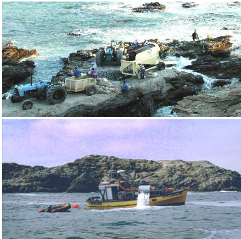
Figure 33: Typical shore-based contractor operation with tractor and classifier parked in the intertidal zone (top) and typical vessel-based diving contractor operating in nearshore areas up to 30 m depth. (Photos: Pisces).
