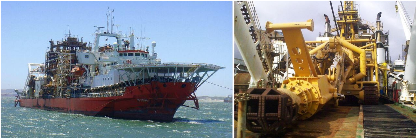
Figure 4: The MV Ya Toivo (left) and its MK2 seabed crawler (right).
