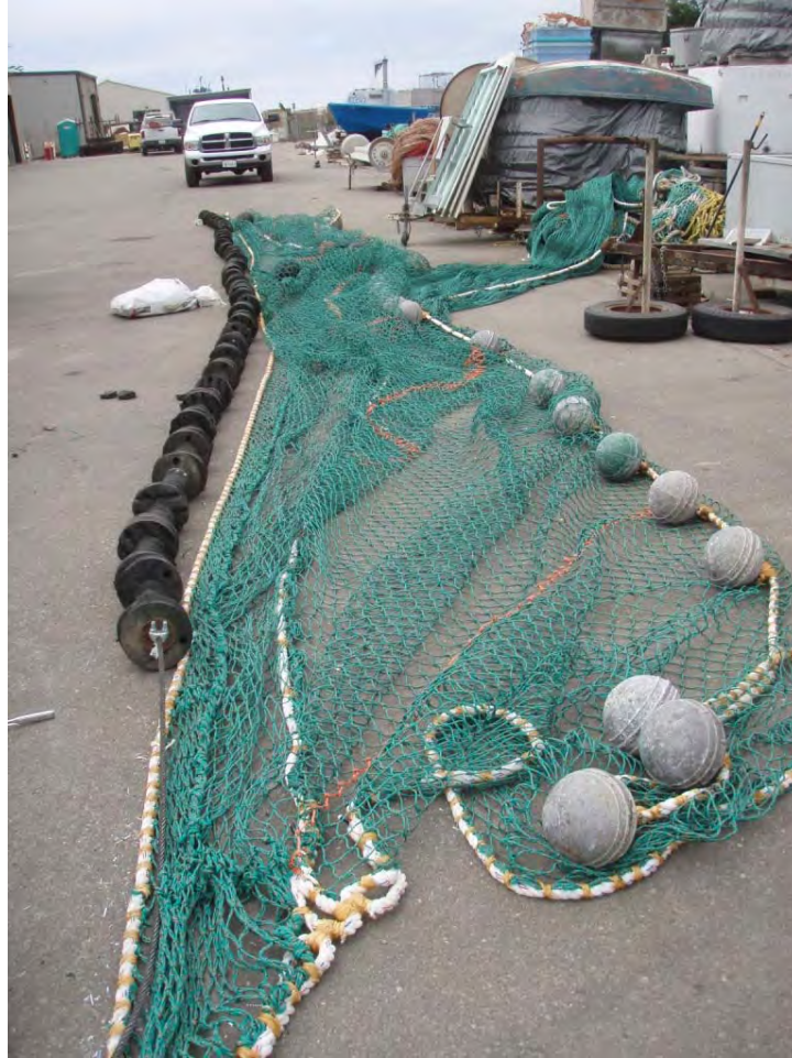
Figure 2. Picture showing the footrope and groundgear (left) and the hearope with attached floats (right).
