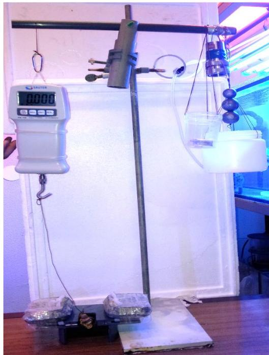
**Figure 7:** The system used to measure the fixation force of the fragments.
