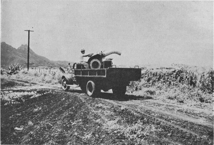
FIGURE 15. A Lawrence mist blower mounted on a truck. Applications of insecticides were made by having one man drive the truck along the periphery of the field while the other directed the spray into the surrounding vegetation.
