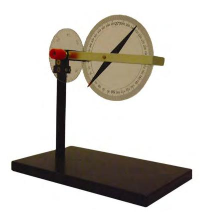
**Introduction:** Dip needles, also commonly known as dip circles, measure magnetic dip. When a magnetic needle is suspended vertically, it will form an angle with a horizontal plane. In effect, the needle represents the exact angle the earth's magnetic field makes at the latitude of the user.
