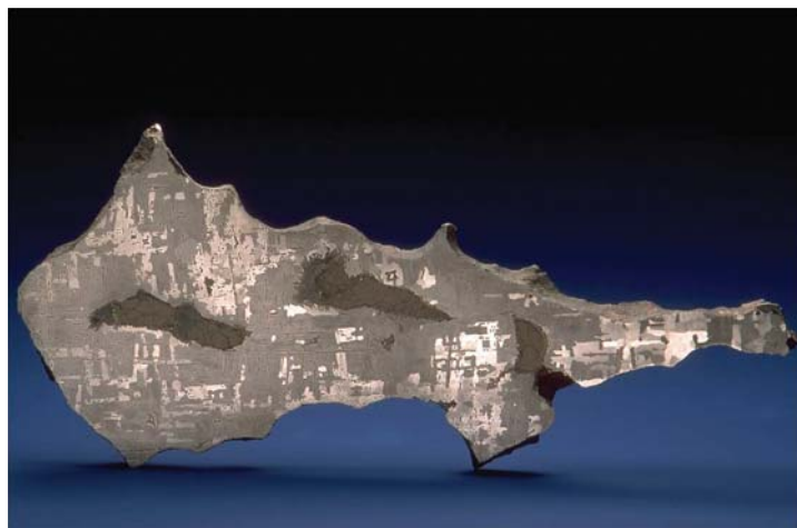
FIGURE 5 The Youndegin IAB meteorite formed from a metallic melt rich in phosphorus, carbon, and sulfur, which cooled and crystallized to form a host of new minerals. The orthogonal texture was formed during slow cooling of the metal, when low-Ni kamacite exsolved from high-Ni taenite. The elongated kamacite lamellae contain cohenite. The dark-colored inclusions are rich in troilite (FeS) and graphite. The specimen is ~40 cm long.
