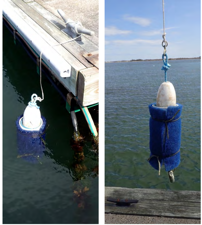
Fig. B. Megalops collector float using an air conditioning filter pad as an artificial settling substrate.
