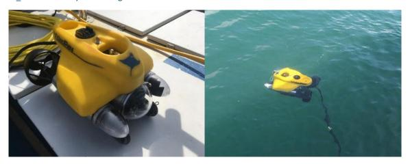
Annex Figure D: VideoRay Pro 4 Remotely Operated Vehicle deployed from R/V Tiger Lily VI
