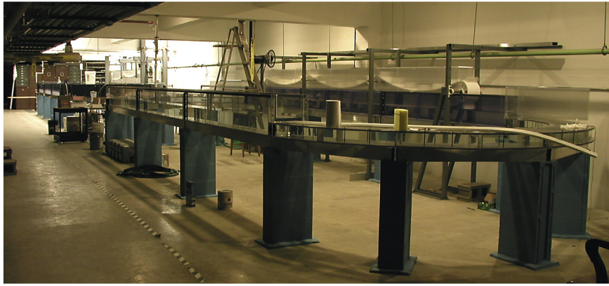
Fig. 5. Indiana University Flume Lab and the flume used for conducting the quartz-silt and quartz-clay-mixed experiments.
