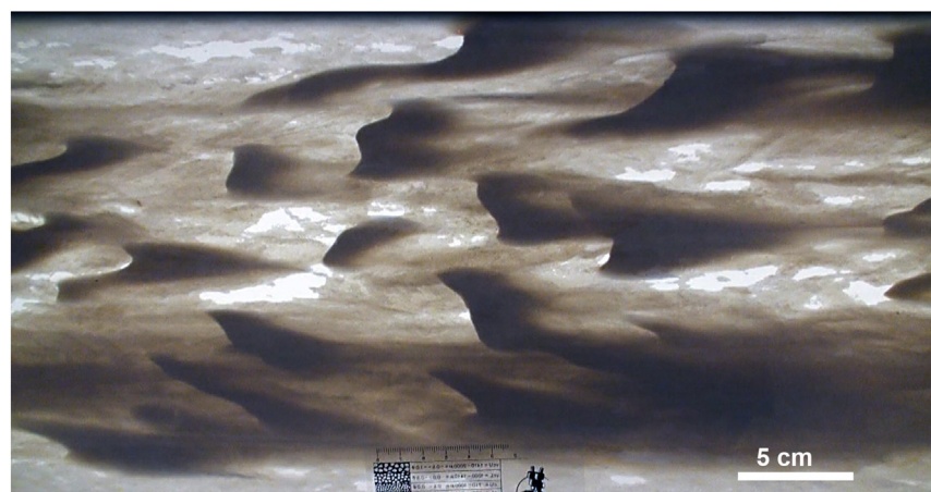
Fig. 14. Migrating ripples in a silt-illite experiment. Flow from right to left, photographed from below. Sediment veneers have covered most of the flume bottom, and with passage of more ripples the bed thickens (becomes darker).
