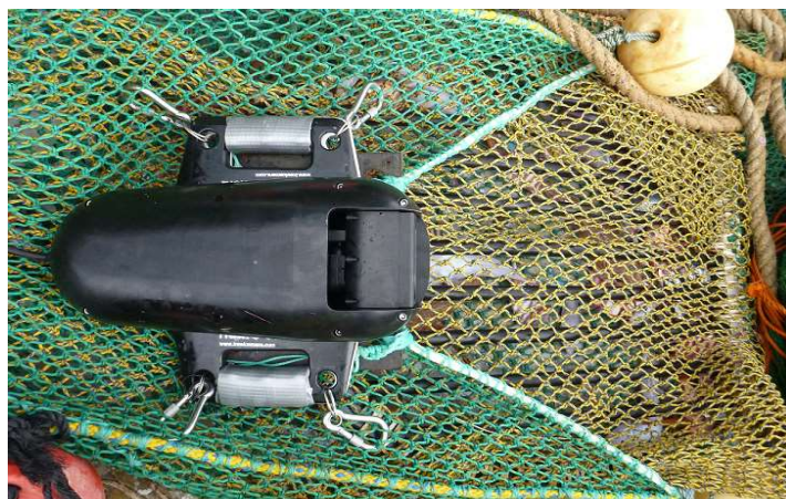
Figure 4. Secondary camera position on 'roof' of net facing rearwards (to the right of the picture). Photo: David Schubert, AFMA
