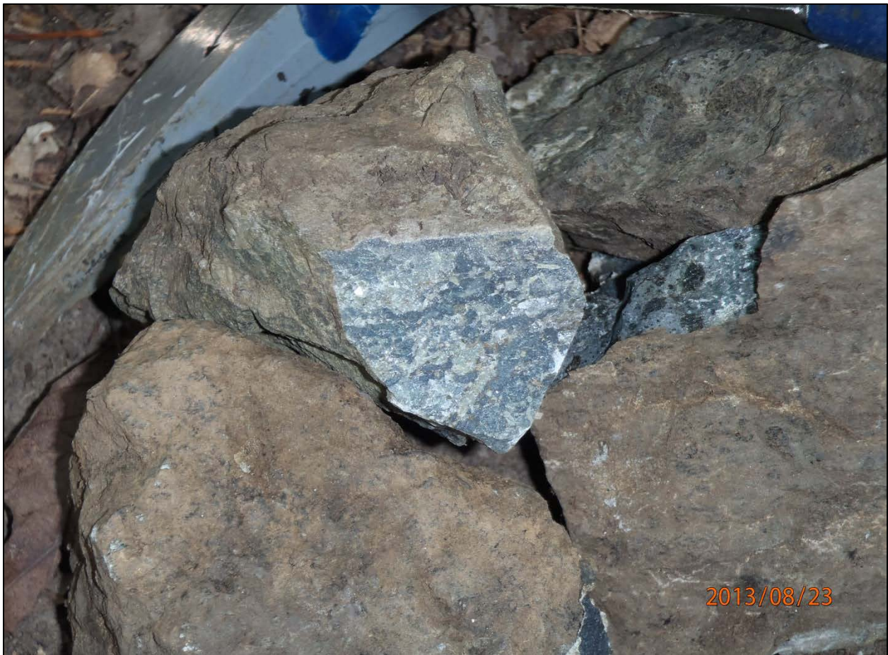
Figure 13. Samples collected at Kidwell #24. Sample in center exhibits marbelization of Bonneterre Formation dolomite country rock. Sample to right shows olivine megacrysts (dark) surrounded by alnöitic groundmass.
