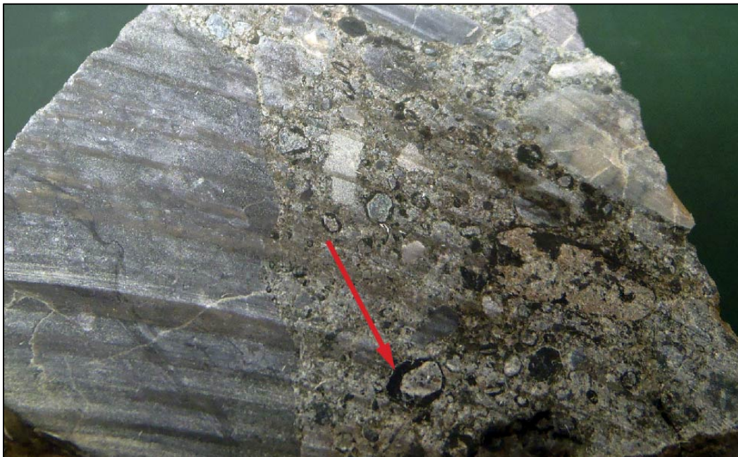
Figure 10. View of sawed specimen shown in Figure 9. This specimen is composed of brecciated county rock surrounded by a groundmass of pelletal lapilli. The pelletal lapilli typically consist of a core surrounded by dark, chloritized igneous material.
