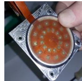
BRIC-LED PDFU Lid showing LEDs.
