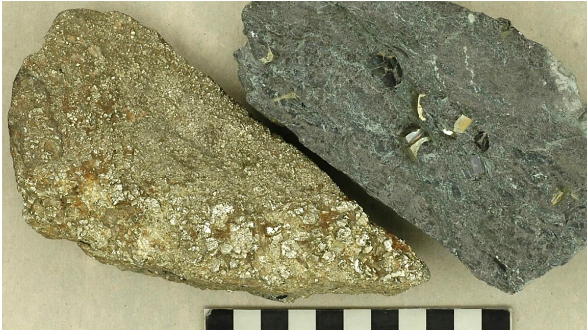
Figure 3.27 – Pyrite ( \text{FeS}_2 ) is a brassy metallic mineral (left; see also Fig. 3.3) with a gray streak color (Fig. 3.2). It can sometimes occur as pentagonal dodecahedral (12 sides, all pentagons) or cubic crystals as is shown here in a metamorphic rock (right). Scale in cm.
