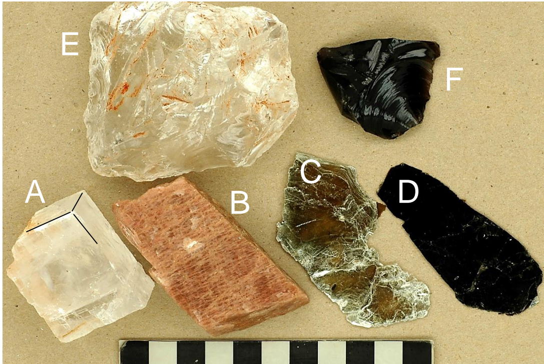
Figure 3.5 –Mineral grains can cleave in several different directions. For example: calcite (A) breaks in three separate directions that have 75° and 105° angles with each other (thin black lines show intersecting edges of different cleavage planes) forming a shape called a rhombohedron or rhomb; feldspar (B) breaks on two planes that are approximately 90° to each other (top surface and left and right sides); muscovite or white mica (C) and biotite or black mica (D) have a single well developed cleavage direction and the mineral easily breaks into thin sheets. Some minerals do not break on flat surfaces but instead form irregular break planes. Quartz (E) forms curved break planes or what are called conchoidal fractures. Natural volcanic glass, a form shown here known as obsidian (F), also has conchoidal fractures that allowed Native Americans to flake the rock into very sharp arrowheads, spear points, and tools. Scale in cm.
