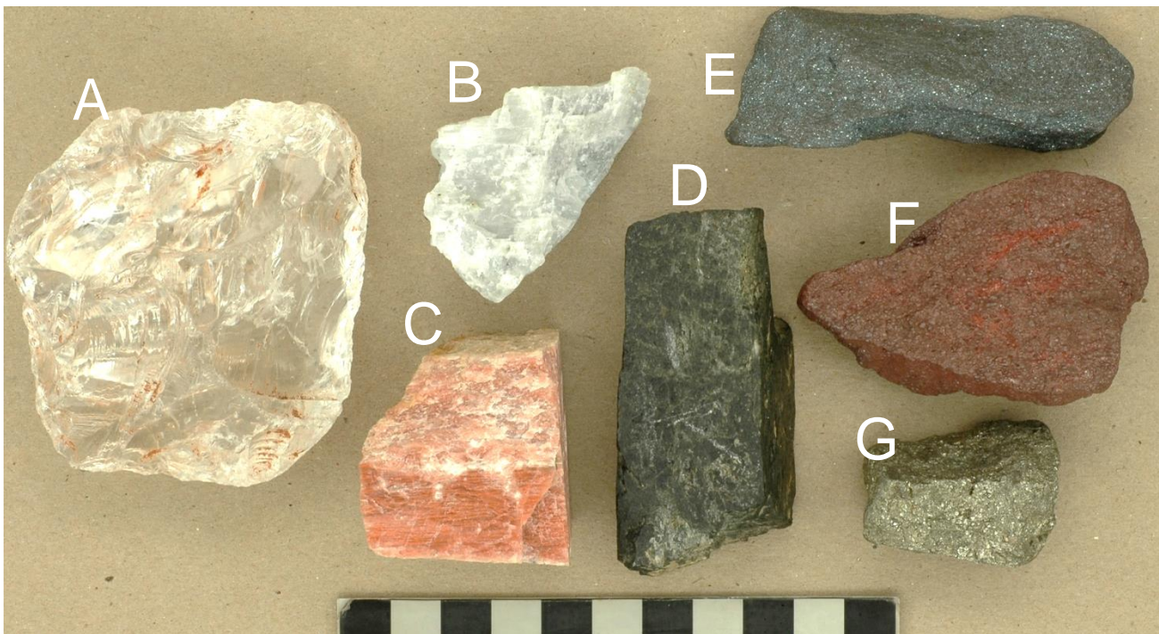
Figure 3.3 – Luster is the overall reflectance and transparency of a mineral. Some minerals are transparent such as quartz (A). Many aluminosilicate minerals are translucent, such as plagioclase feldspar (B), alkali feldspar (C), and pyroxene (D). These minerals are translucent when viewed in thin pieces. Oxide and sulfide minerals (E-G) are opaque. Opaque minerals may have a high surface reflectivity such as specular hematite (E) which is metallic bluish gray. Fine-grained hematite has an earthy opaque luster (F). Pyrite (G) is metallic brassy yellow. Scale in cm.
