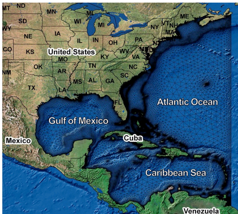
Figure 2.70 ADCIRC Model Mesh Telescoping from the Western North Atlantic Ocean, Caribbean Sea and Gulf of Mexico into the Lower St. Johns River (Hagen, et al. 2006)
