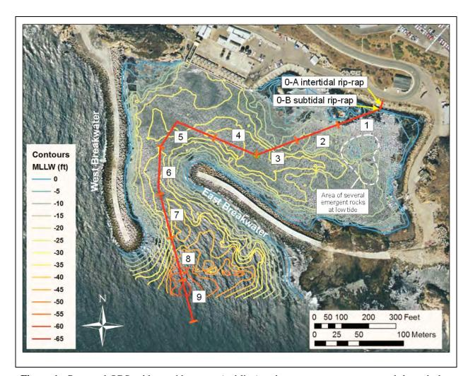
**Figure 1.** Proposed OBS cable corridor route (red line) and transect segments surveyed through the DCPP intake cove on May 17–20, 2011. Depth contours are from multi-beam hydroacoustic surveys conducted in 2005.
