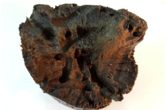
Fig. 5: a cross section of a piece of wood with moderate presence of S. annandalei .
