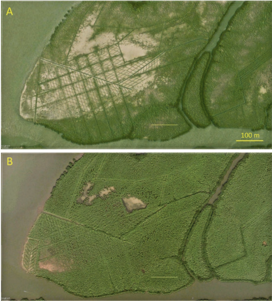
Fig. 10.3 Hydrological restoration implemented in mangrove wetlands in Pichavaram, Tamil Nadu, India, showing original main and feeder channels excavated circa 1996. (a): March 3, 2003; (b): January 29, 2016 (Source: Google Earth Pro; image area: 55.5 ha; eye altitude 881 m; Latitude: 11^{\circ}25'59.86'' N, longitude: 79^{\circ}47'28.89'' E at the center of the images)
