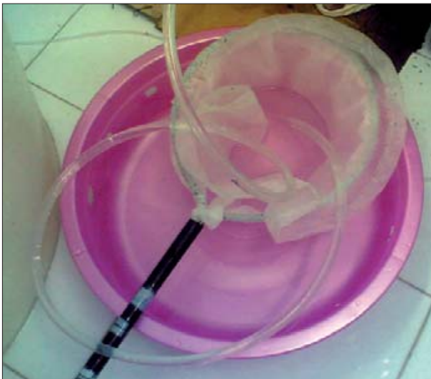
Figure 1. Sieving the tank water through a filter.
