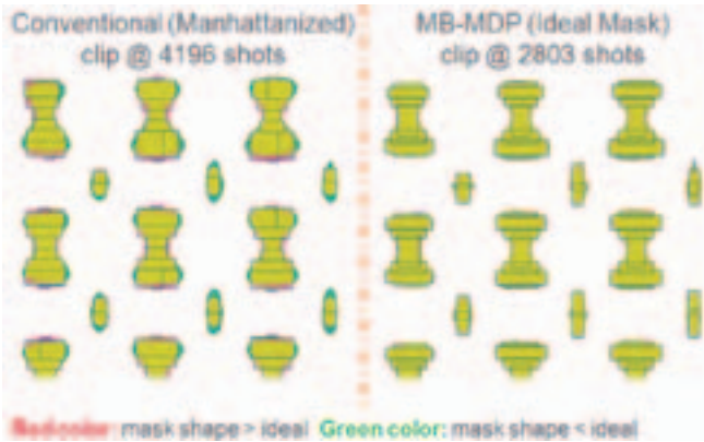
Figure 15. Mask shape comparison at 33% shot count reduction.
