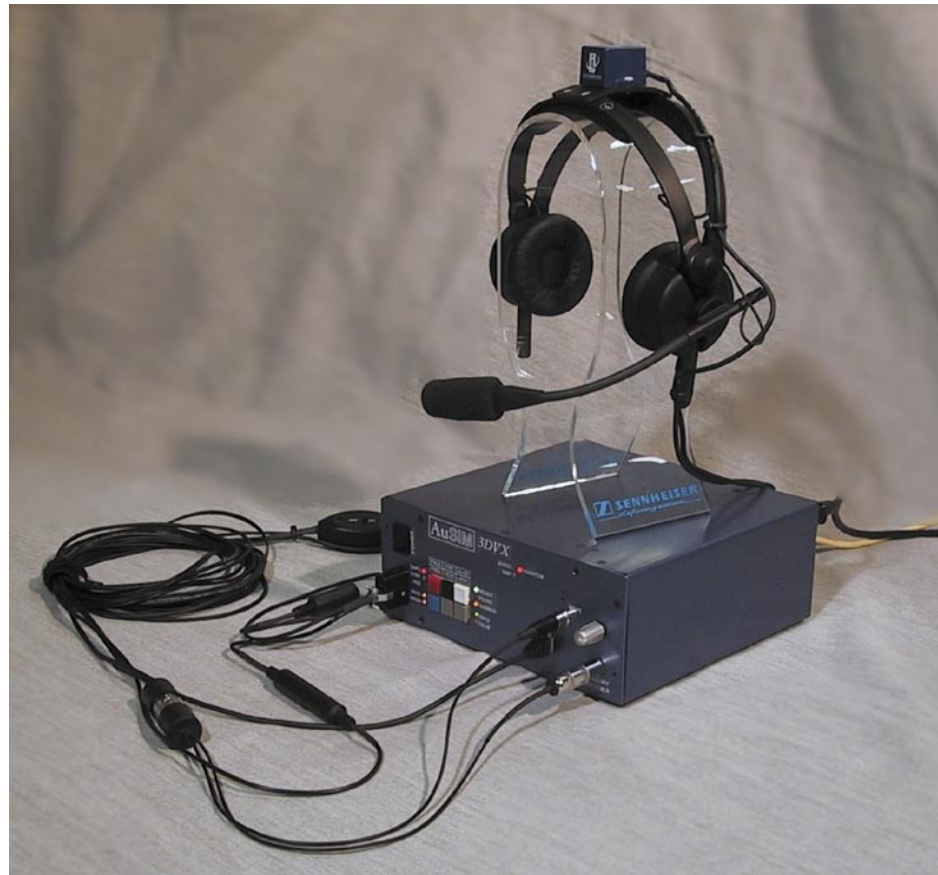
The 3-D Voice Communication Interface System, AuSIM, Inc.'s latest hardware product, connects to a network via ethernet. Each participant uses one system, and the headset is tracked in orientation and global position. Derivatives of this system are being developed for wearable and vehicle applications.
