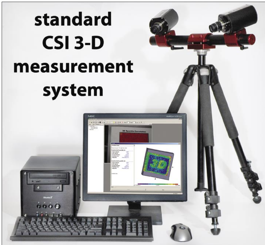
Correlated Solutions, Inc.'s three-dimensional measurement system utilizes two digital cameras and associated hardware to obtain pairs of stereo images.
