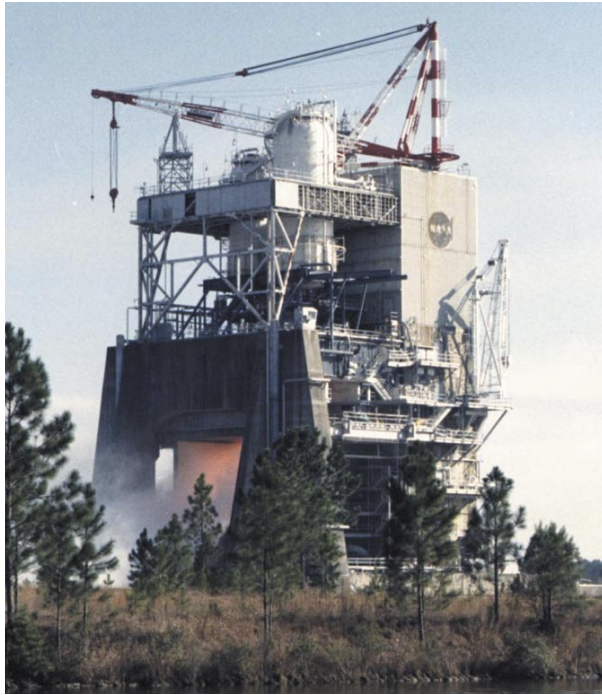
A Space Shuttle Main Engine undergoes a test firing on the A-1 Test Stand at Stennis Space Center.
