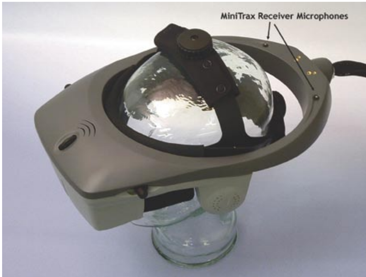
InterSense's immersive headsets, like this NVIS Head Mounted Display, bring 3-D to life when integrated with IS-900 MiniTrax 6-DOF Inertial-Acoustic Tracking Technology.
