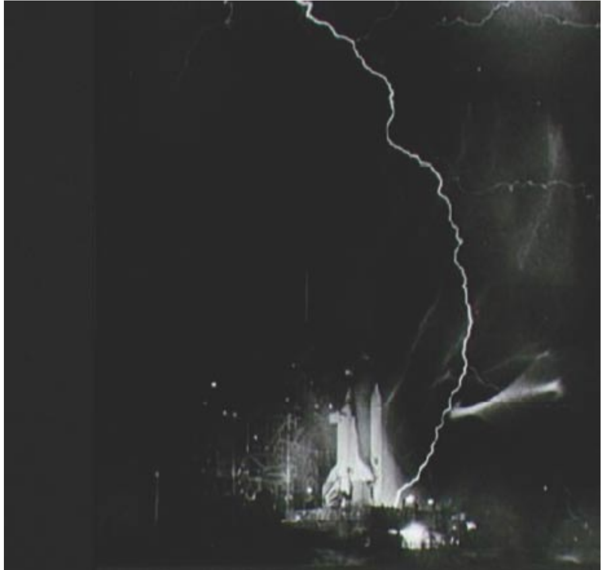
NASA created this technology to determine the strike location of lightning around the launch pads so that crews could test the wires and electrical components after a storm.
