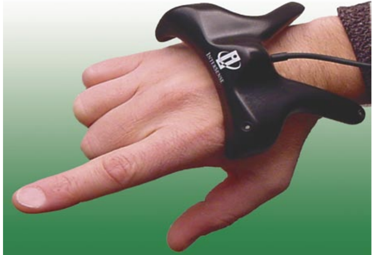
Virtual reality systems depend on motion-tracking sensors to relay information between the user and the computer. Pictured here is the InterSense IS-900 MiniTrax 6-DOF Hand Tracker for immersive environment interaction.
