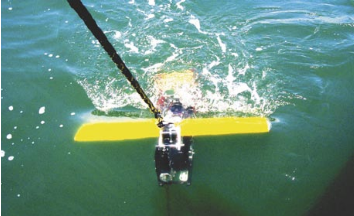
The DOLPHIN “swims” behind research vessels and samples the water to validate satellite imagery. It provides valuable information about ocean color and quality.
