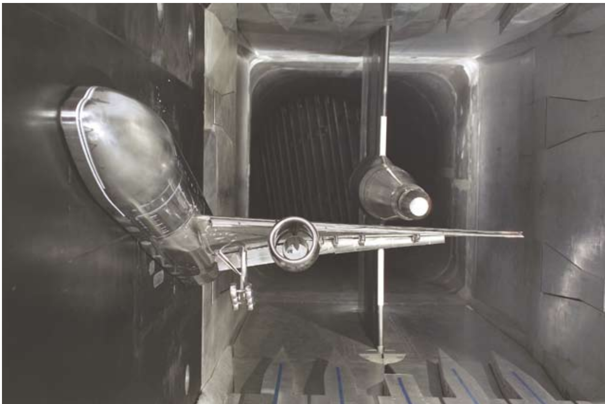
Wing trailing edge design concepts for Boeing's new 787 aircraft are being tested on a 5.2-percent scale 777 semi-span model inside Langley Research Center's National Transonic Facility.
