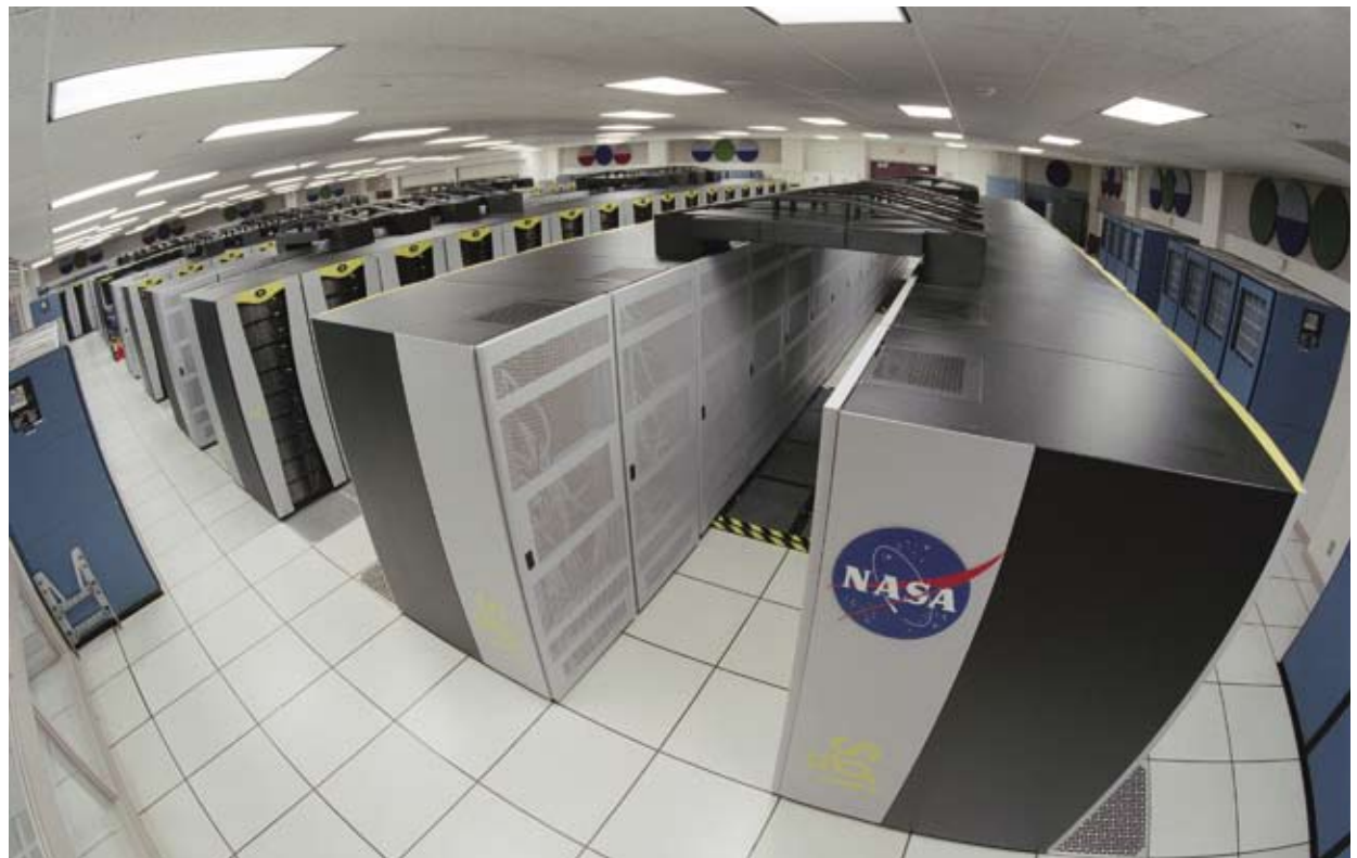
A bird's-eye view of the 10,240-processor SGI Altix "Columbia" supercomputer located at Ames Research Center. While Columbia is helping NASA achieve breakthroughs and solve complex problems in support of its missions, it has also been made available to a broader national science and engineering community.
