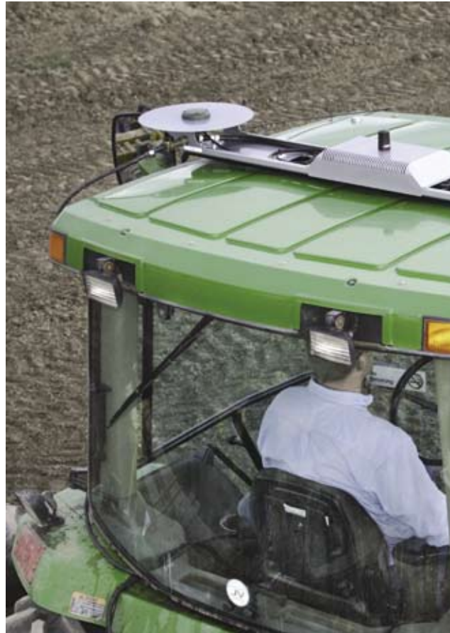
RTK AutoSteer helps farmers reduce fuel costs, decrease driver fatigue, and eliminate overlap. Pictured here are GPS system antennas roof-mounted on a farming tractor and the touchscreen controls for the GPS guidance system installed in the cockpit.
