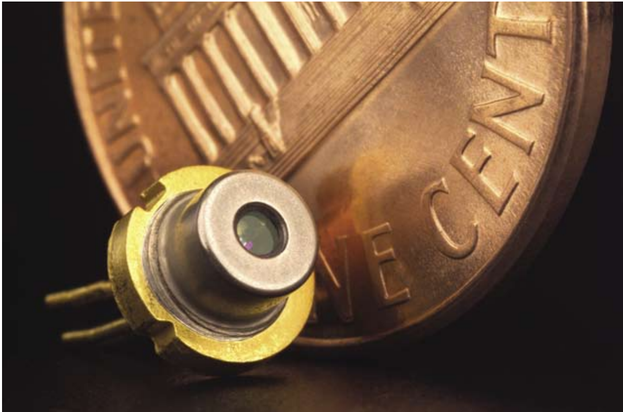
Miniaturized tunable diode laser packaging for sensing and measuring atmospheric water vapor.
