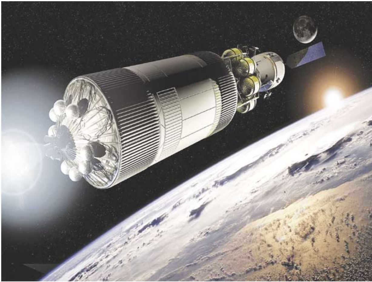
A rocket fires for translunar injection, carrying the Crew Exploration Vehicle and lunar lander toward the Moon.
