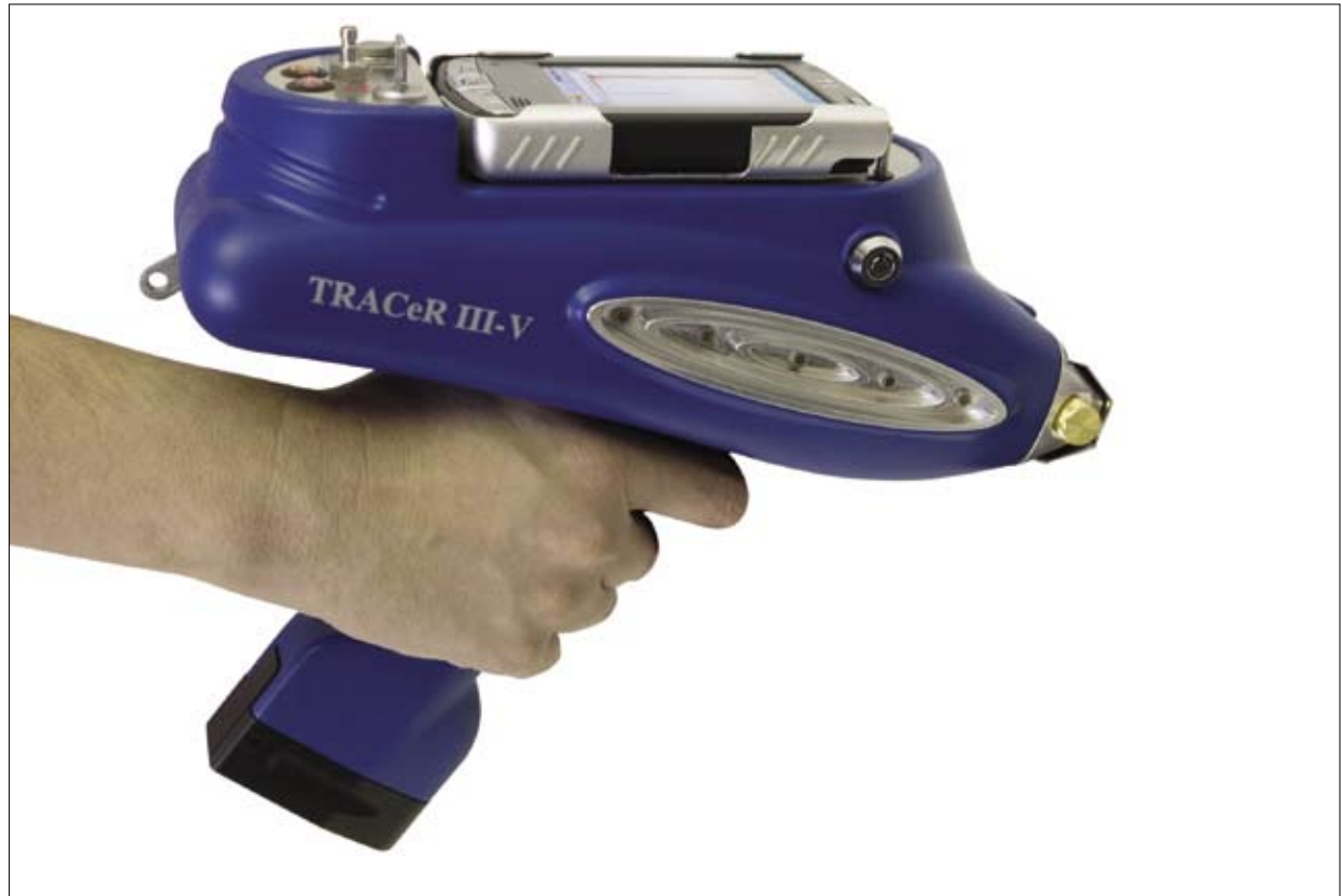
KeyMaster Technologies, Inc.'s TRACeR III-V portable, hand-held scanner, for detecting and tagging unique elemental codes. This instrument was designed to help NASA evaluate parts destined for the space shuttle.
