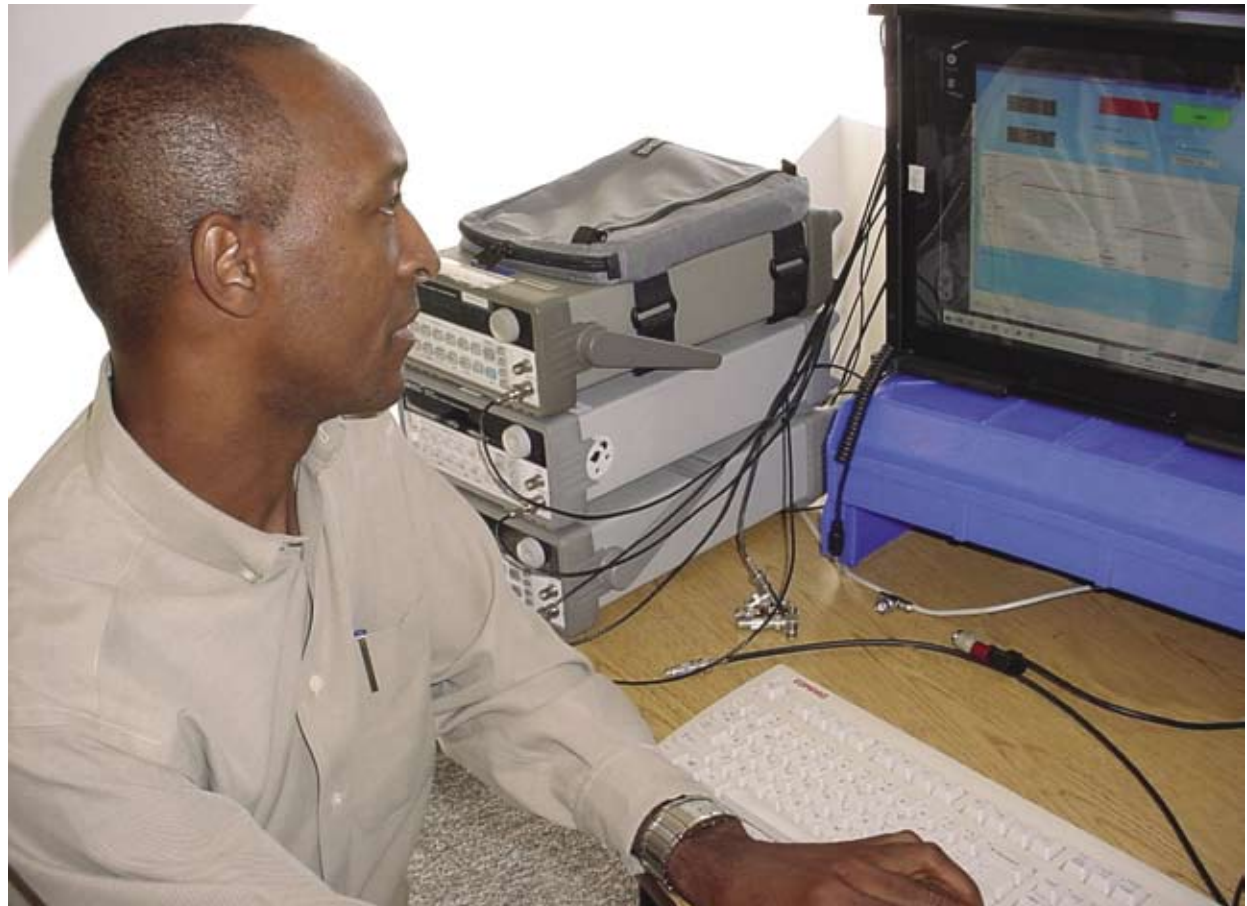
An Ophir Corporation engineer works with a ground-based unit that provides air data for air vehicles, as well as information for turbulence detection and wind profiling.
