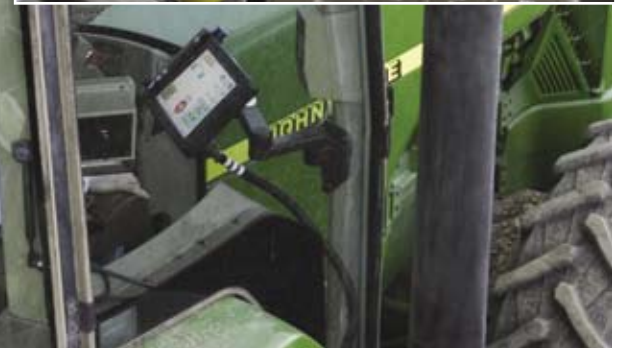
RTK AutoSteer helps farmers reduce fuel costs, decrease driver fatigue, and eliminate overlap. Pictured here are GPS system antennas roof-mounted on a farming tractor and the touchscreen controls for the GPS guidance system installed in the cockpit.
