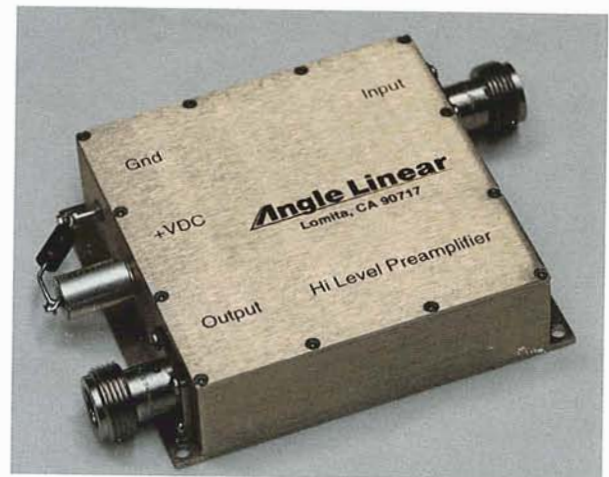
Originally developed for NASA Space Shuttle communications, Angle Linear's receiving preamplifier has a very sensitive high dynamic range. The system is used in a variety of communications applications, including business, government, tracking, and cellular.
