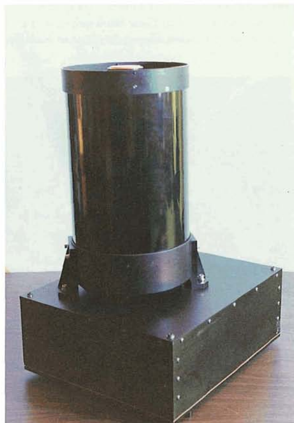
Science and Engineering Services, Inc.'s Micro Pulse Lidar System resulted from NASA research and patents. This instrument is employed to make detailed measurements of atmospheric constituents and is available on the commercial market.
