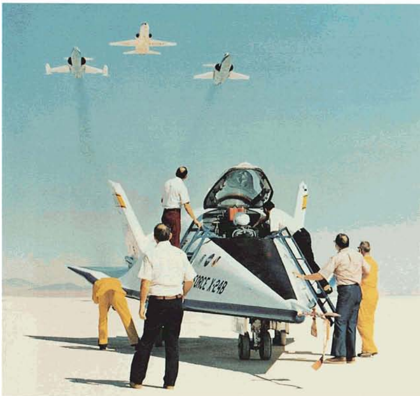
The X-24B is surrounded by support personnel on Rogers Dry Lakebed after a research mission as two F-104s and a T-38 fly overhead. First flown at NASA Dryden in 1973, the X-24B demonstrated the ability for a pilot to maneuver and safely land an unpowered craft on a conventional runway, as the Space Shuttle does today.
