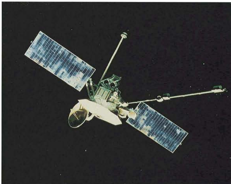
Mariner 10, launched on November 3, 1973, was the first to use "gravity-assist," using the gravity of one planet to slingshot a spacecraft onward to another. The innovative technique has been applied to many spacecraft missions over the years, with more being planned.
