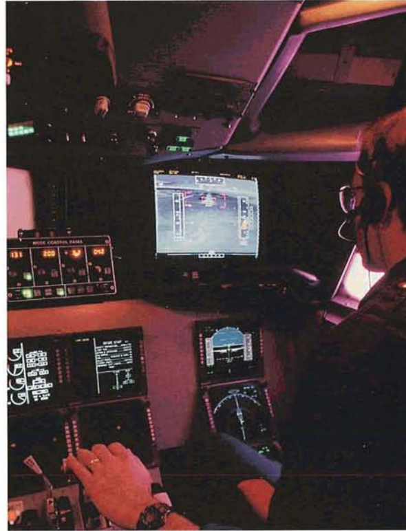
A NASA pilot makes a "windowless landing" aboard a NASA 737 research aircraft in flight tests aimed at developing technology for a future supersonic airliner. Cameras in the nose of the airplane relay images to a computer screen in the otherwise blind research cockpit.
