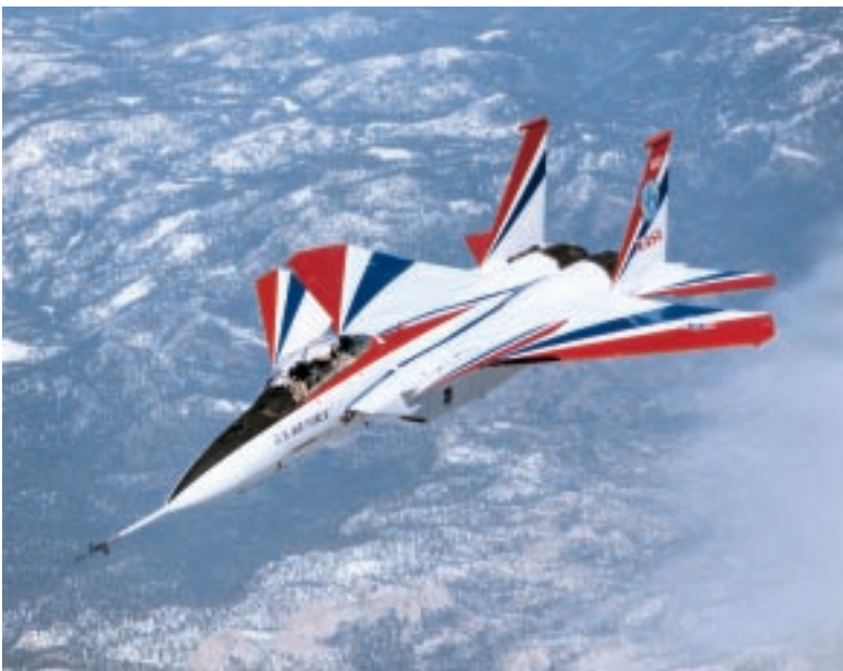
NASA's Advanced Control Technology for Integrated Vehicles (ACTIVE) F-15 aircraft has been highly modified for testing control system technologies, including engine thrust vectoring. Flown by NASA's Dryden Flight Research Center at Edwards Air Force Base, California, the aircraft is heavily instrumented for its research role, including state-of-the-art avionics and cockpit displays.
