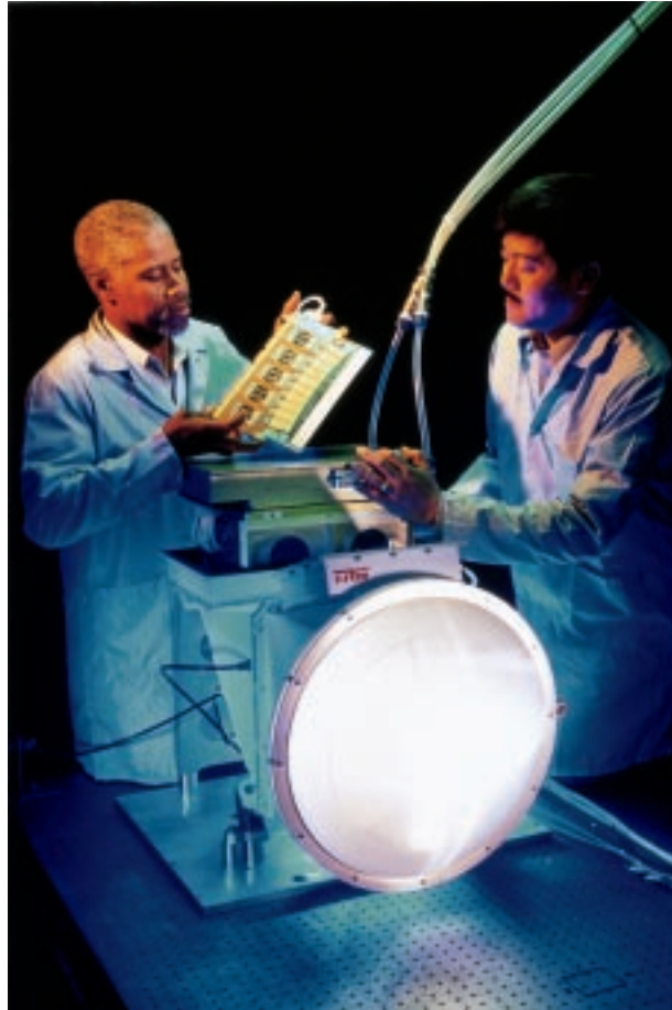
Engineers inspect a passive millimeter wave camera, a weather-piercing camera designed to "see" through fog, clouds, smoke, and dust. NASA Langley is working with a TRW-led industry consortium and the Department of Defense on the project.
