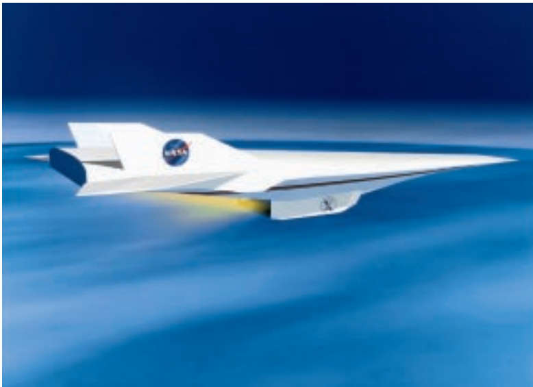
Hyper-X program features testing of unpowered aircraft that will fly up to ten times the speed of sound (7,000 mph) to demonstrate "air-breathing" engine technologies.
