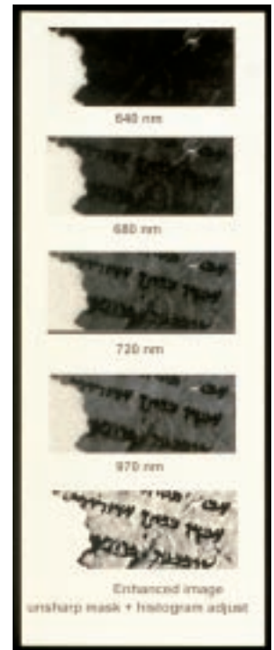
Never-before-seen writing on the Dead Sea Scrolls was uncovered by coupling liquid crystal tunable filter technology to an imaging spectrometer.
