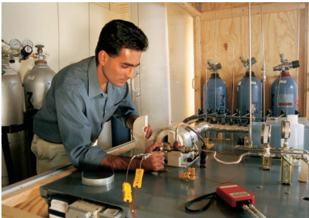
Dr. Paul Menacherry, a PCI research and development engineer, is working with a custom-built test rig used to simulate automotive exhaust gas.
