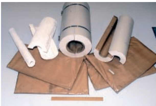
Blankets of aerogel materials act as phenomenal insulators. NASA-supported research has stirred commercial interest in the product for a variety of business and consumer applications.
