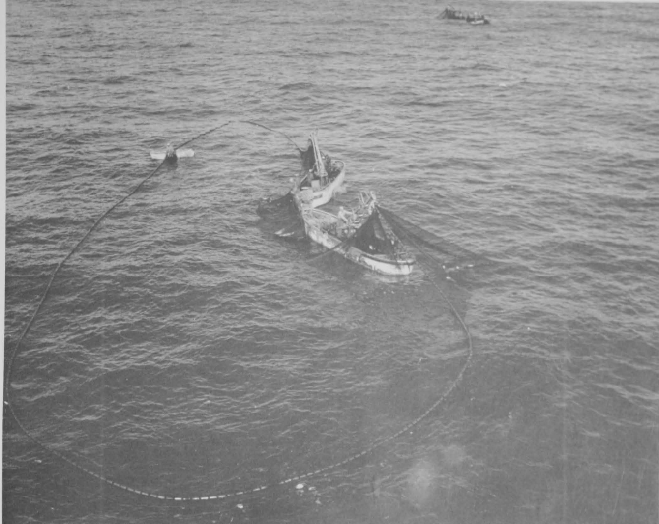
Figure 4.--Purse seine boats using hydraulic blocks to concentrate the catch into the bunt of the net.
