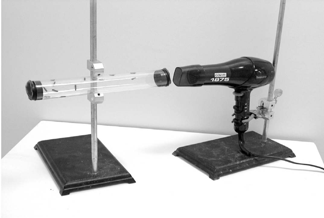
Figure 1. Airflow apparatus used to induce desiccation stress in gravid female H. coagulata .
