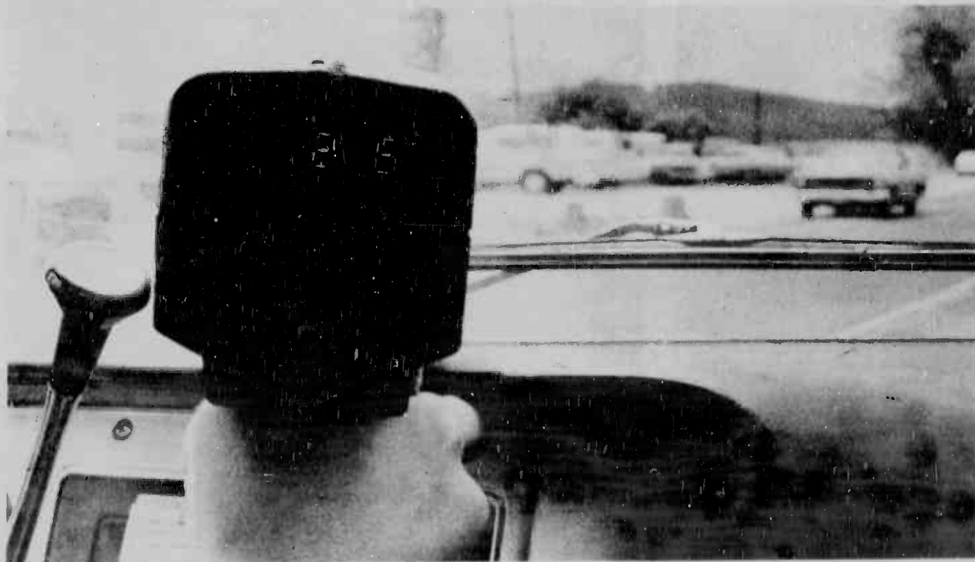
ATTENTION ON THE ROAD — Motorists aboard the Air Station may find a pistol-shaped apparatus pointed at them from military police trucks. It's the new radar gun now employed by station MPs to combat speeders on base. The gun is much more precise since it fires a narrower beam than conventional radar.
