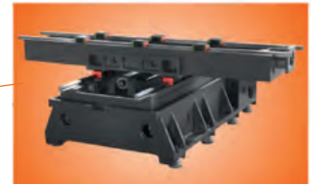
X and Y construction axis
