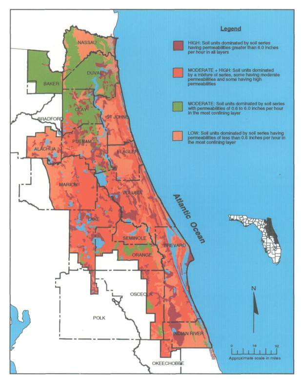
Figure 10. Susceptibility of soils to dewatering
