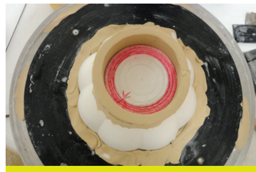
1 The teapot body, solid cast in plaster from a found object. A cottle at the top will form the lid.
