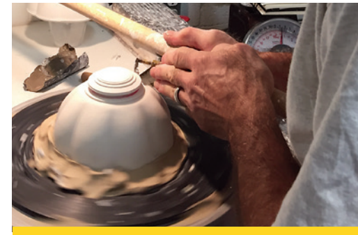
2 The lid is turned using the potter’s wheel as a vertical lathe.
