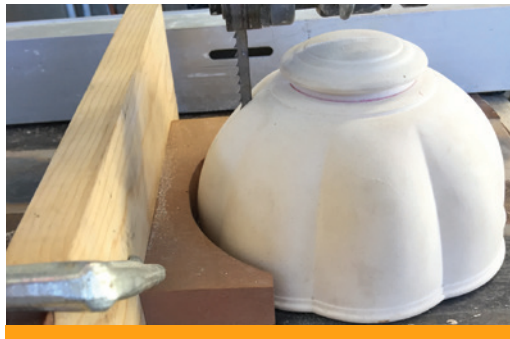
3 The model is cut using a custom band saw jig; then handle and spout forms are added.
