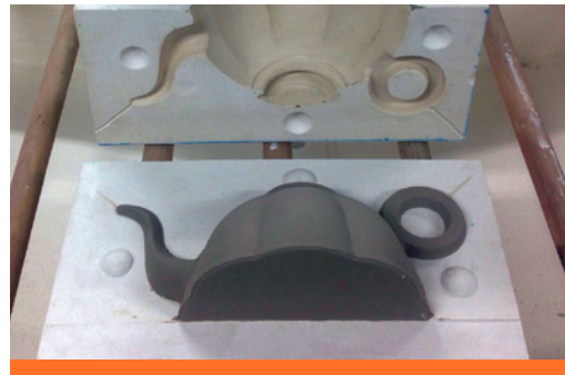
4 A three-part mold is made, then used cast the form in porcelain.
