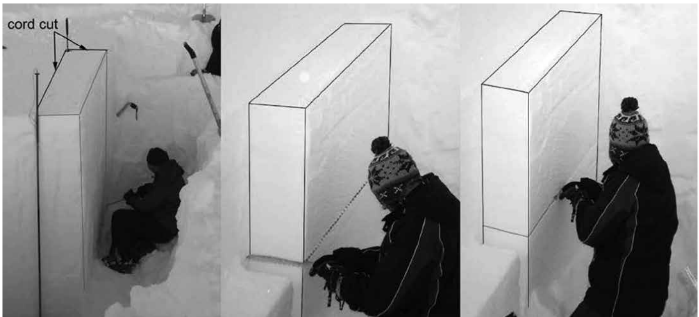
FIGURE 2.17 The PST process (left to right): isolating the column with probes and cord; identifying the weak layer and preparing to cut; dragging the saw along the weak layer until the onset of propagation. Lightly brushing the weak layer with a glove or brush before cutting helps the operator follow the layer along the column. (P: ASARC)
