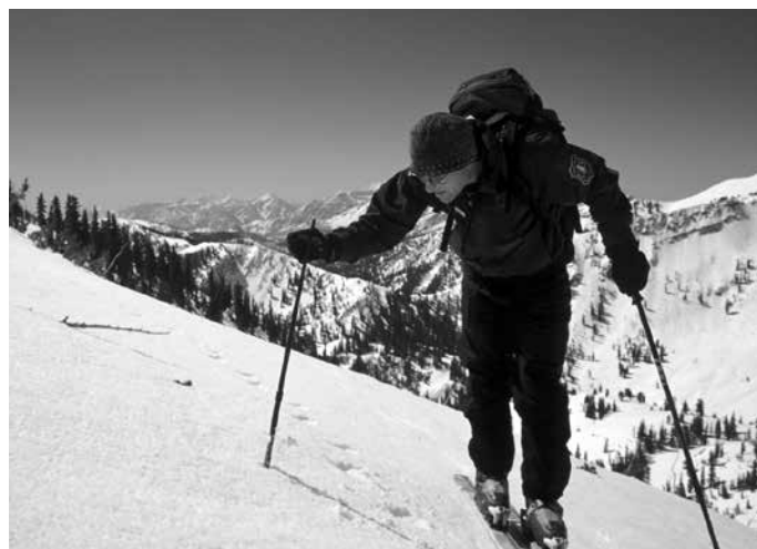
FIGURE 2.20 The ski pole poke, aka Ski Pole Penetrometer. (P: Bruce Tremper)
