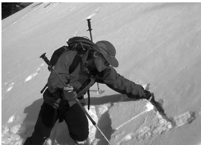
FIGURE 2.19 A hand shear test. (P: Bruce Tremper)
