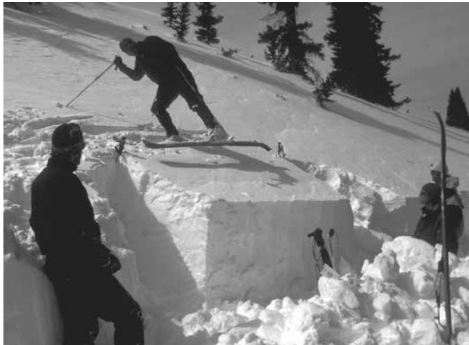
FIGURE 2.11 Stepping onto the block during a Rutschblock Test. (P: Kelly Elder)
