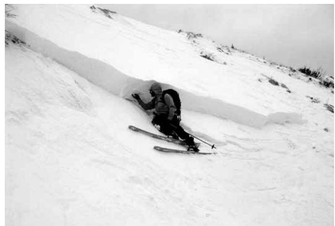
FIGURE 2.2 Different types of snow profiles clockwise from left: Full Profile, Test Profile, Fracture Line Profile. Snow profiles will vary depending on the information needed to support a particular application. (P: Karl Birkeland, Bruce Tremper, and Ben Pritchett)
