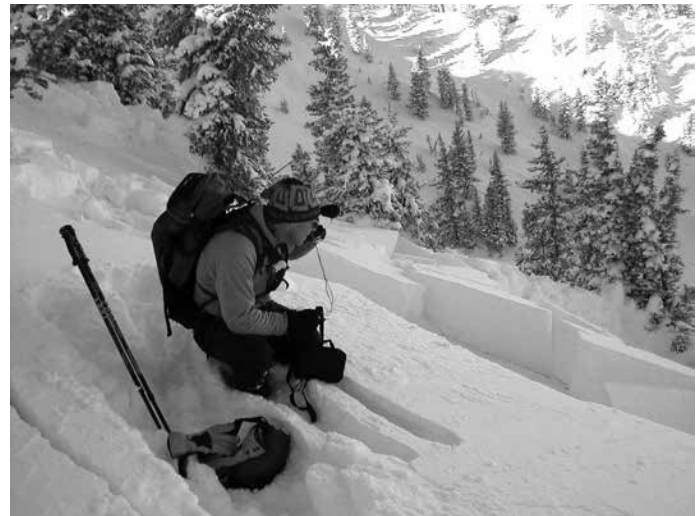
FIGURE 3.2 Measuring the slope angle of a slab avalanche. (P: Bruce Tremper)
