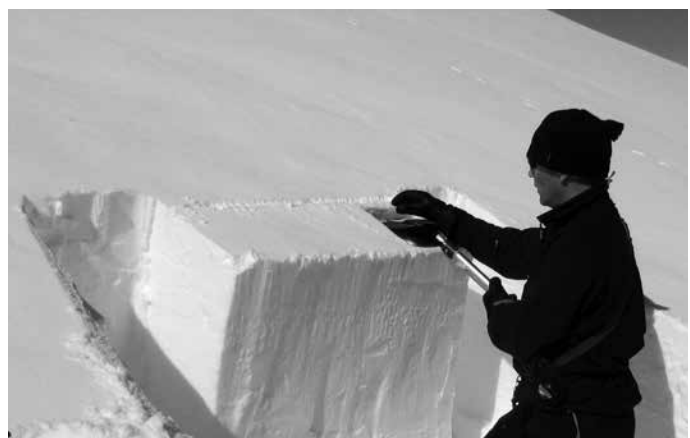
FIGURE 2.15b and c Schematic and photograph of the Extended Column Test. (P: courtesy of Ron Simenhois)
