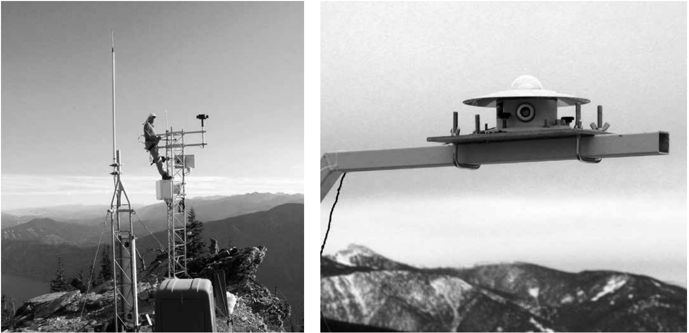
FIGURE D.5 Left: An exposed wind site to monitor general atmospheric flow. (P: Mark Moore) Right: A pyranometer for measuring incoming short wave solar radiation. (P: Don Sharaf)
