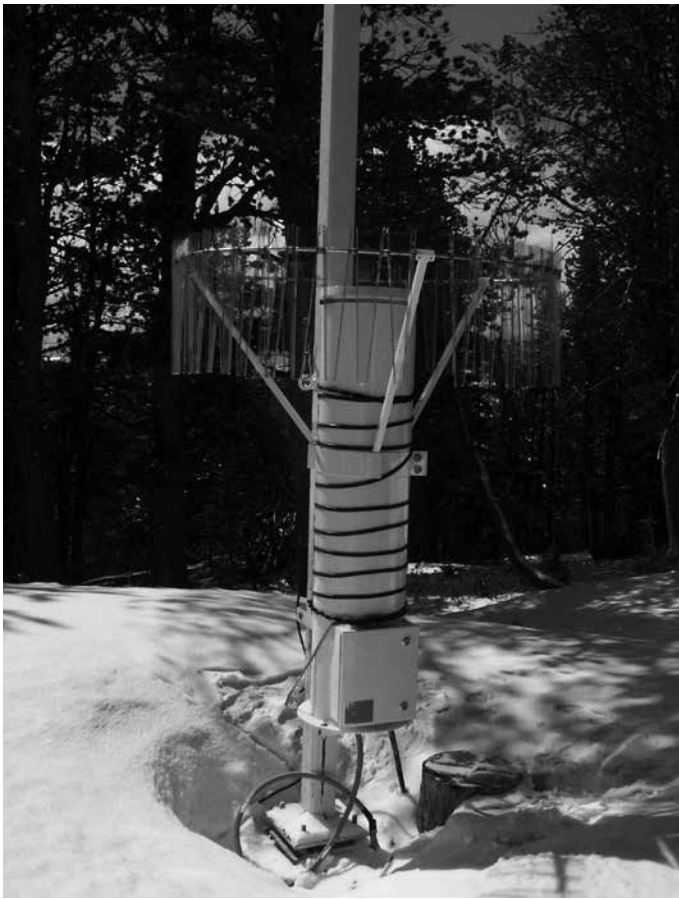
FIGURE 1.4 Precipitation gauge with Alter shield. (P: Tom Leonard)
