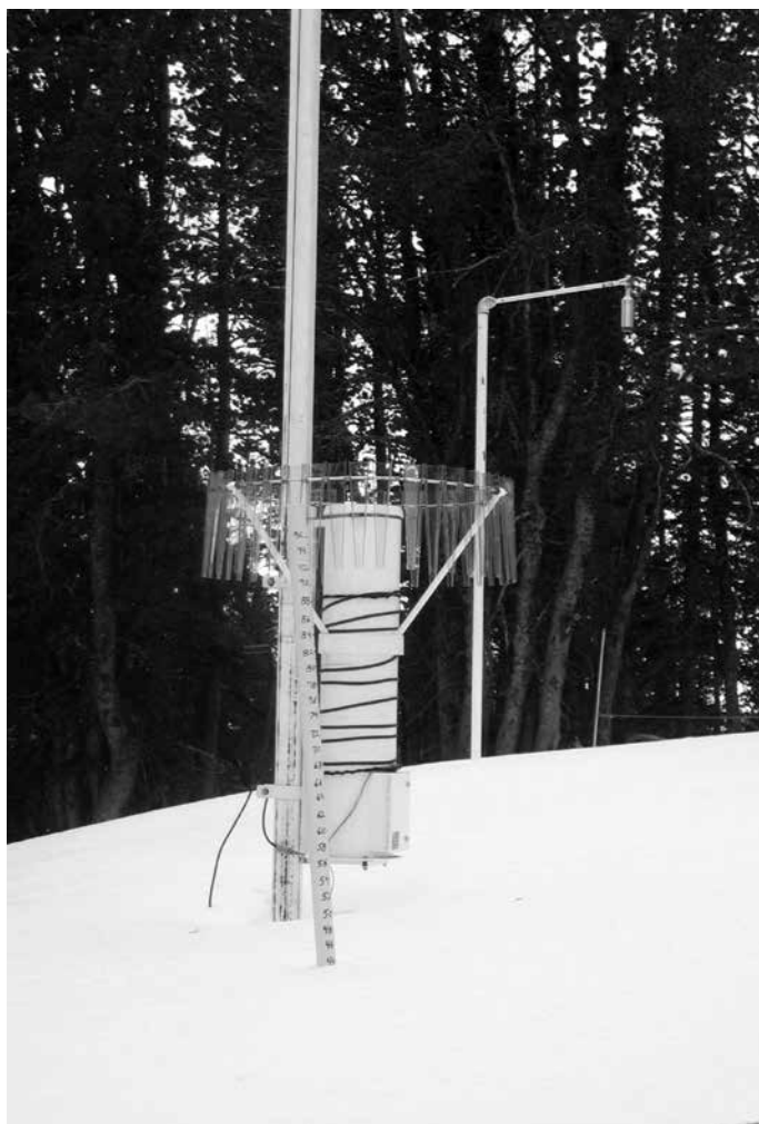
FIGURE D.3 A manual snow stake, precipitation can, and ultrasonic snow depth sensor. (P: Don Sharaf)
