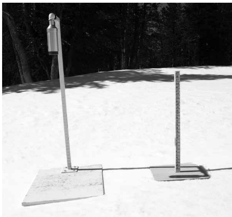
FIGURE 1.3 Left: Snow board graduated in centimeters. Right: Automated snow board and snow board graduated in inches. (P: Tom Leonard)
