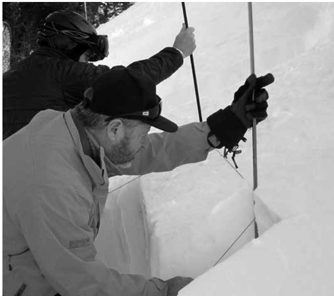
FIGURE 2.15a Cutting an ECT (P: courtesy Don Sharaf)
