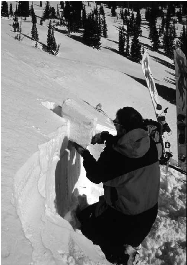
FIGURE 2.21 The Shovel Tilt Test. (P: Howie Garber)
