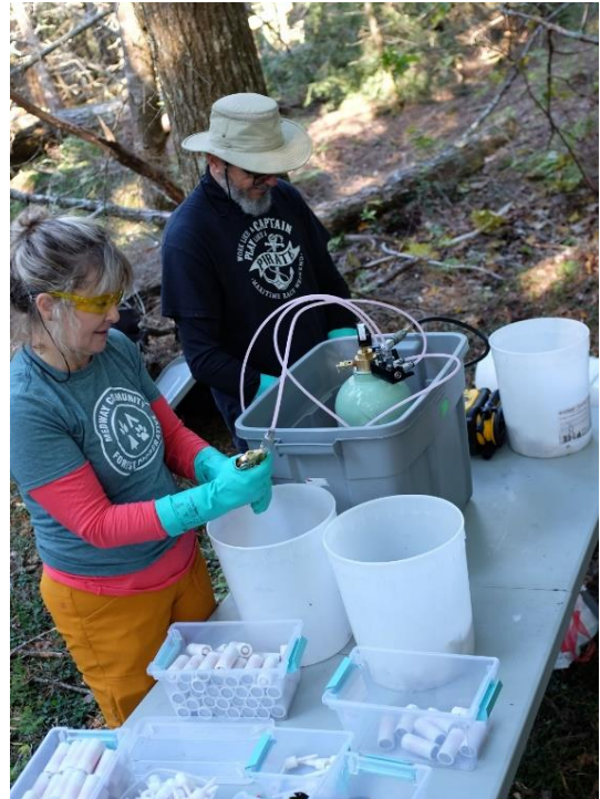
Filling table showing filling tank and canisters-all contained against spillage.
