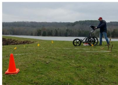
Figure 3. Collecting GPR data at Site 1 along Ferne Clyffe lake.
