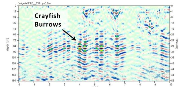
Figure 7a. 2D vertical GPR profile at Site 2 at Vancil Farm near Du Quoin, IL.
