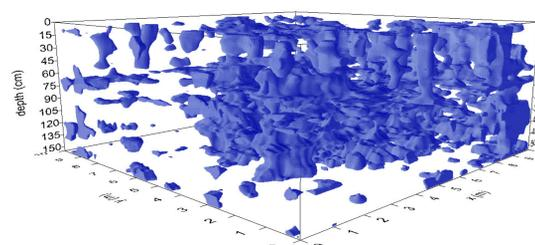
Figure 6c. Isosurface (3D model) of GPR data at Site 1 near Ferne Clyffe lake.
