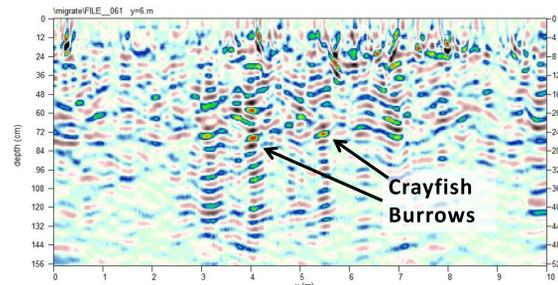
Figure 6a. 2D vertical GPR profile at Site 1 near along Ferne Clyffe lake.
