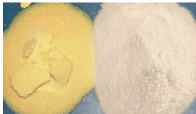
Comparison of the tendency of vitamin A powder to form lumps after 1 hour of storage at 80 % relative humidity and 35°C (right side ELCOvit A 250, left side the product used for comparison).
