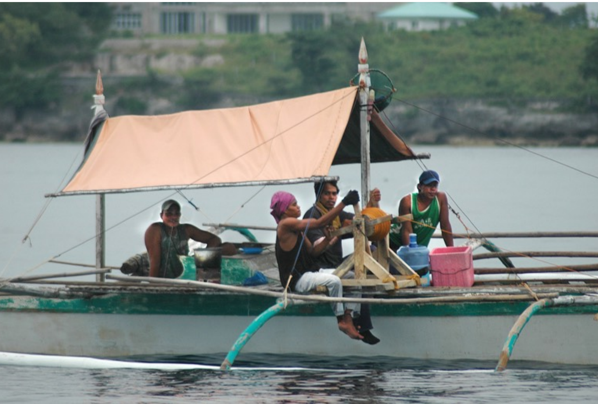
The rope for this depth is about 500 m long, and several men are required to get the small dredge on board.
