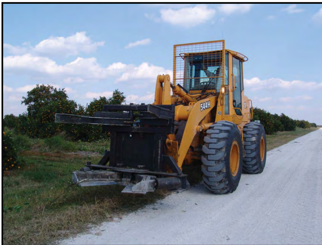
Figure 1: Front-end loader used in clipping citrus trees with tree shear attachment.
