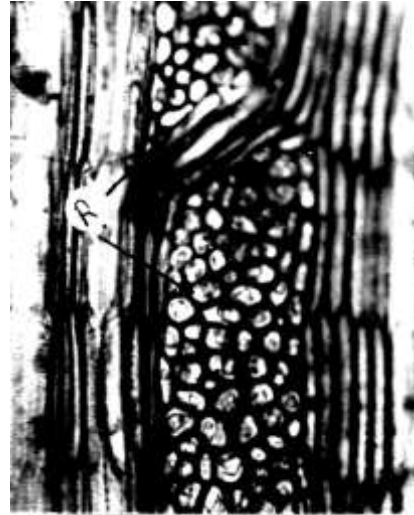
L.S. in Tamarix tetragyna (x125), showing ray (R) < 2 mm high, ray width 5-12 cells; ray frequency < 4/ \text{mm}^2
