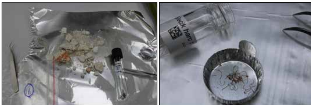
Figure 10: Mortar Sample Sampled (a), Sample of Completed Physical and Chemical Cleaning Process (b).
