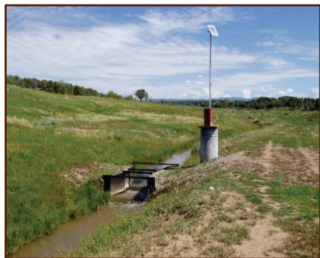
A network of telemetry linked gages provide real-time ditch flow measurement on portions of the Pine River Indian Irrigation Project.
